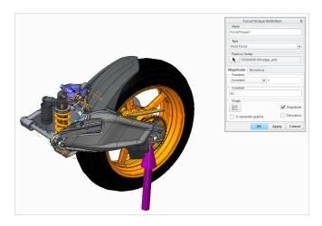
Dynamic forces are applied to the assembly using PTC Creo MDO to optimize quality.
